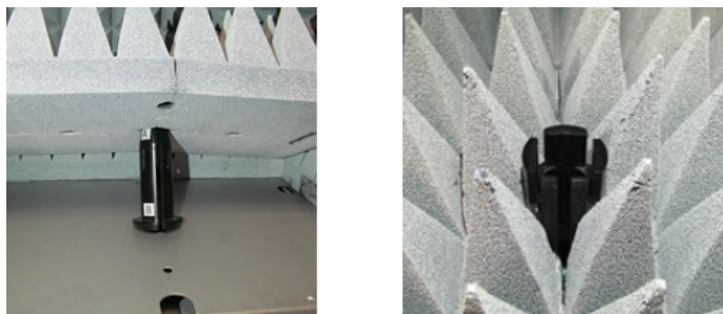
Figure 4-5: Mounting adapter B with the help of adapter A (here shown without the RF cable)
