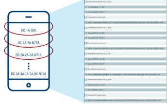
The R&S®CM sequencer Shuffler iterates through device MRDC band combinations. This provides a fully automated way of checking the health of the DUT.
