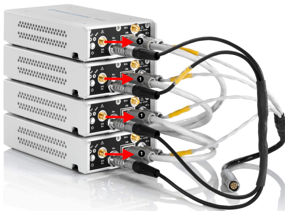
Figure 3-14: LAN cable connected to LAN connectors of 4 R&S TSME6 devices
