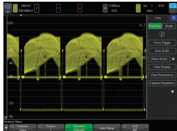
Figure 26: Triggering on 1080p HDTV signal analysis.
