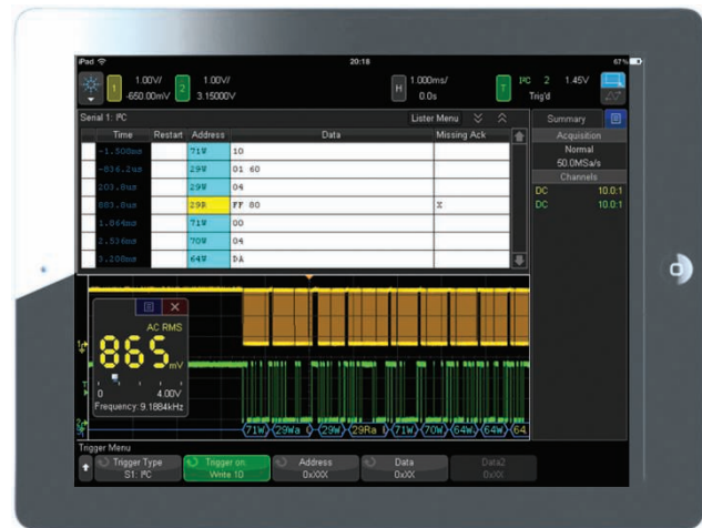
Figure 37: Tablet virtual front panel control.
