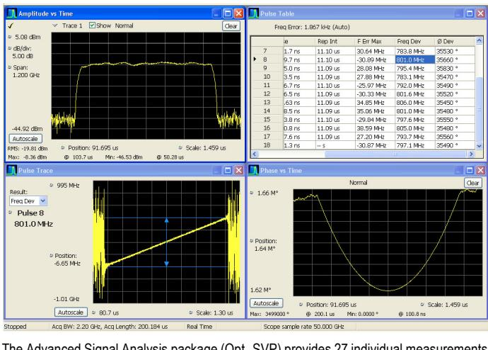
The Advanced Signal Analysis package (Opt. SVP) provides 27 individual measurements to automatically characterize long pulse trains. An 800 MHz wide LFM chirp centered at 18 GHz is seen here with measurements for pulses 7 through 18 (upper right). The shape of the pulse can be seen in the Amplitude vs. Time plot shown in the upper left. Detailed views of pulse #8's frequency deviation and parabolic phase trajectory are shown in the lower two views.
