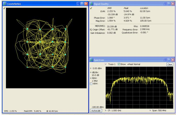
Wideband satellite and point-to-point microwave links can be directly observed with SignalVu analysis software. Here, General Purpose Digital Modulation Analysis (Opt. SVM) is demodulating a 16QAM backhaul link running at 312.5 MS/s.
