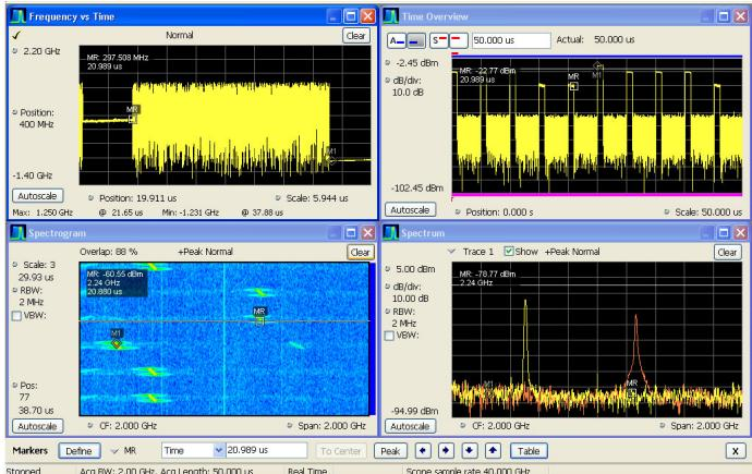
Time-correlated, multidomain view provides a new level of insight into design or operational problems not possible with conventional analysis solutions. Here, the hop patterns of a narrowband signal can be observed using Spectrogram (lower left) and its hop characteristics can be precisely measured with Frequency vs. Time display (upper left). The time and frequency responses can be observed in the two right-hand views as the signal hops from one frequency to the next.
