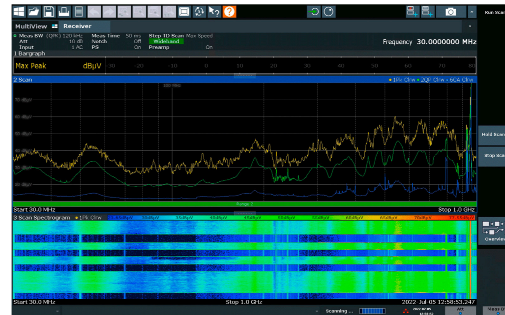
Receiver measurement with CISPR detectors from 30 MHz to 1 GHz in one single segment with R&S®ESW-B1000 bandwidth extension option with real-time spectrogram.
