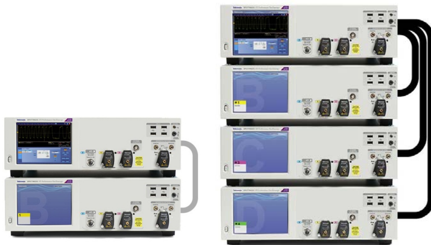
Figure 5: Multiple DPO70000SX units can easily be connected together (up to four total) to scale up performance and capabilities as testing needs change.
