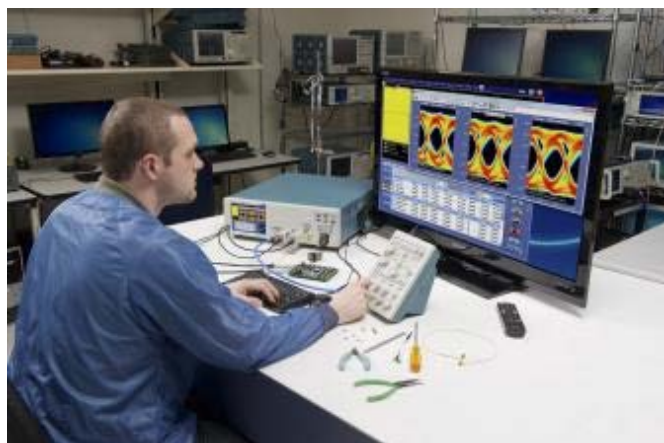
Figure 2: High Speed Differential Serial Bus Measurements using DPO70000SX Oscilloscope with remote panel and large monitor.
