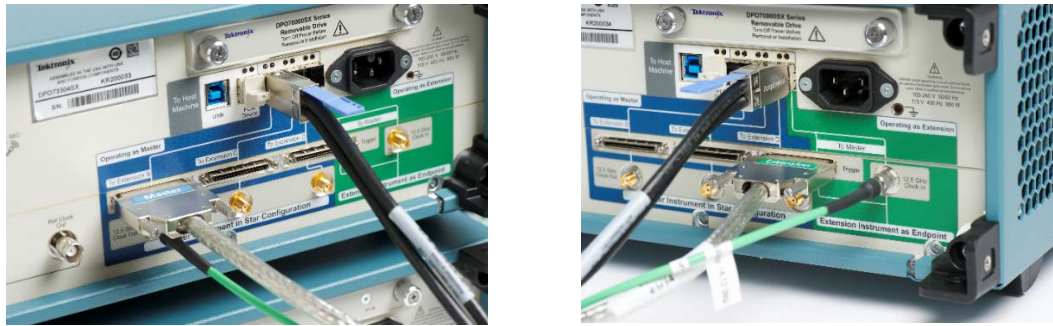
Figure 4: UltraSync Master and Extension unit connections showing sample clock reference, trigger bus connection, and high-speed data connections.
