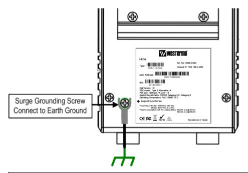
Note: 1. Ensure the Surge/Lighting is well connecting with Chassis Grounding 2. Remove the Surge /Lighting Screw, before performing Insulation / Hi-pot Testing.
