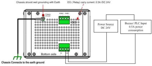
Digital Output Wiring simulate Diagram
