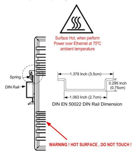
Follow the steps below to mount PMI Managed Switch to the DIN-Rail track:
