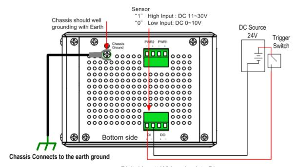
Digital Inputt Wiring simulate Diagram
