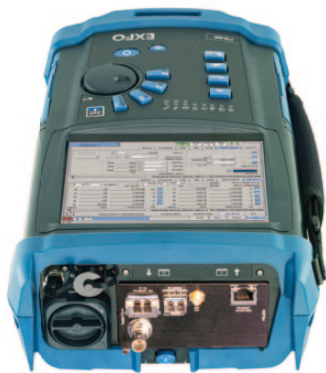
The FTB-8525/8535 Packet Blazer modules can be housed in the FTB-200 Compact Platform.
